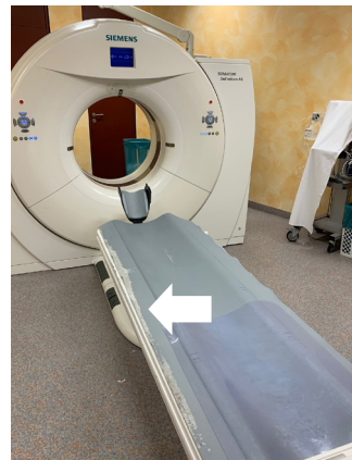
Figure 1: Illustration of mechanical damage (arrow) of the patient mattress on the CT with severe wear of the flaps on the right side due to frequent patient transfer.
