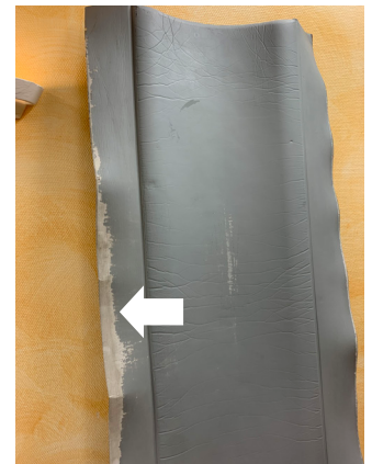
Figure 1: Illustration of mechanical damage (arrow) of the patient mattress on the CT with severe wear of the flaps on the right side due to frequent patient transfer.
